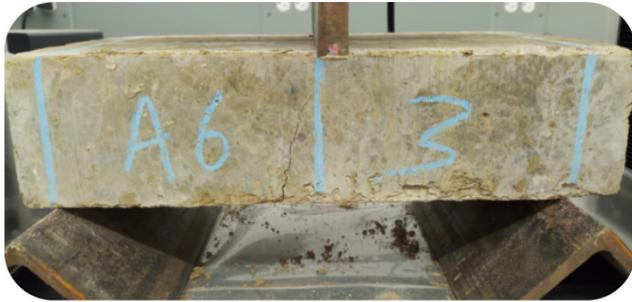
*Flexure test of unreinforced earth block*
