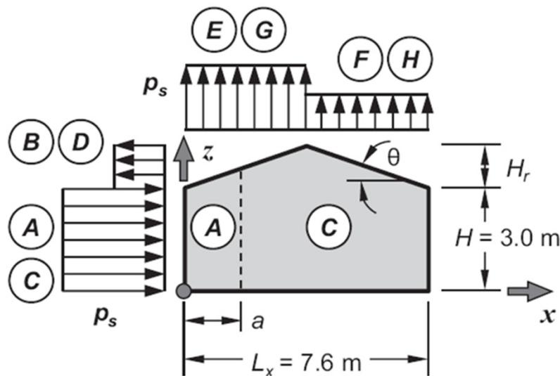
*Schematic representation of wind pressures on MWFRS (Matta et al. 2015)*
