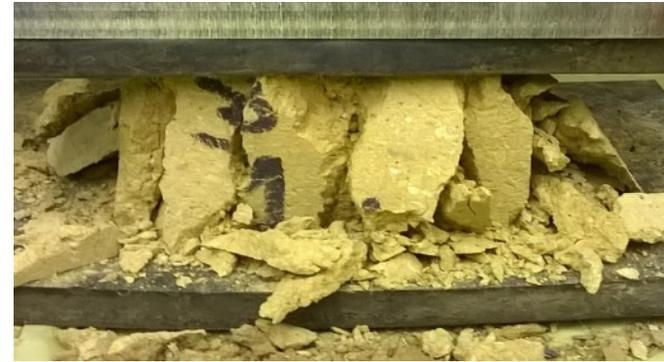
*Specimen after compression test*
