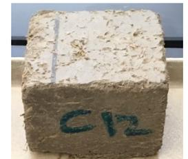
Specimens after durability test
