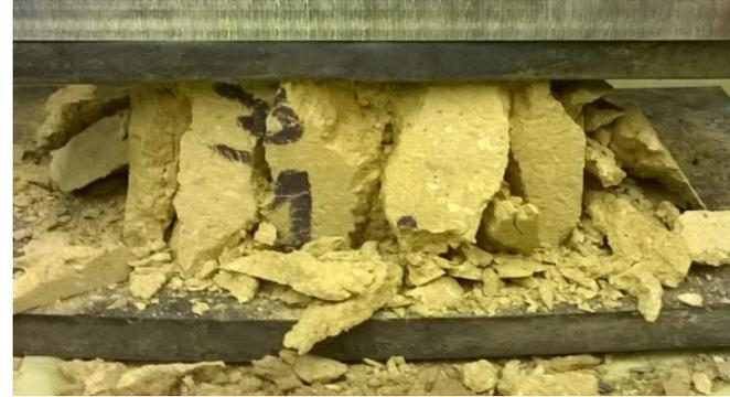
*Specimen after compression test*
