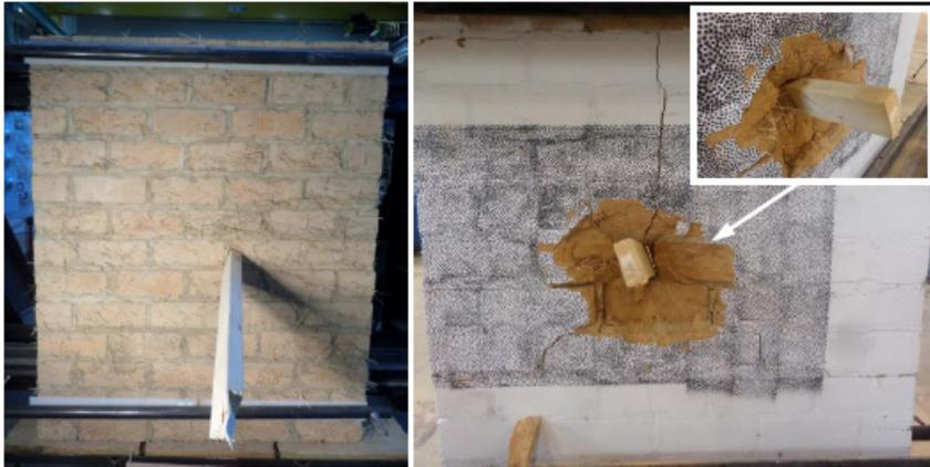
*Windborne debris impact resistance of earth block walls (Cuéllar-Azcárate MC 2016)*
