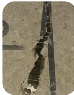
Crack pattern in SBF-reinforced earth block
