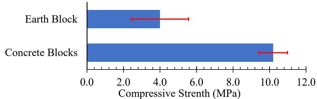
*Variability in compressive strength of different masonry materials*
