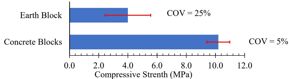
*Variability in compressive strength of different masonry materials*
