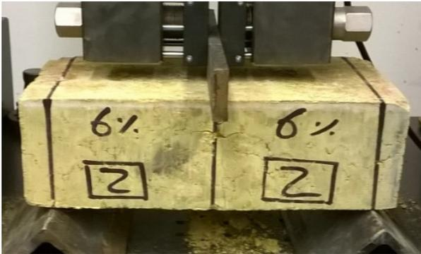
*Specimen after flexure test*
