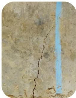
Crack pattern in unreinforced earth block
