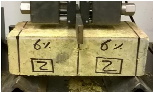
*Specimen after flexure test*
