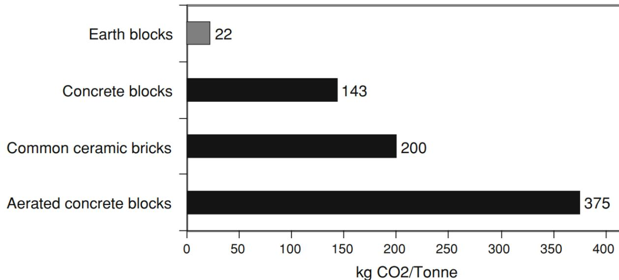
*Embodied carbon in different masonry materials (Morton et al. 2005)*
