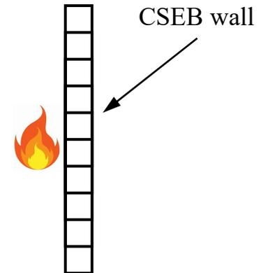
*One sides of CSEBs wall expose to time-temperature profile*
